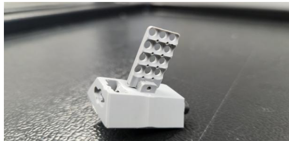
3D Printing in resolutions below 10 \mu\text{m} (Picture: Andreas Roser)
