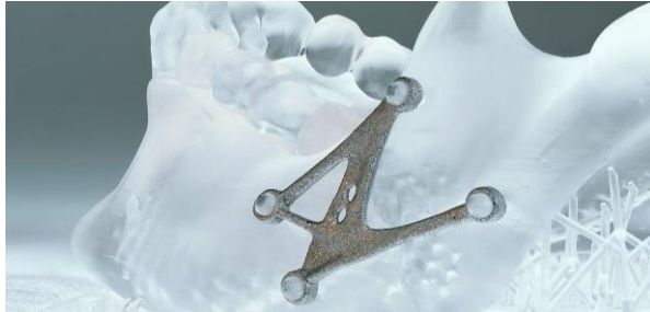
Personalised titanium-implant, designed using automated modeling within MIRACLE II (Picture: Dr. Reinhard Wendler)
