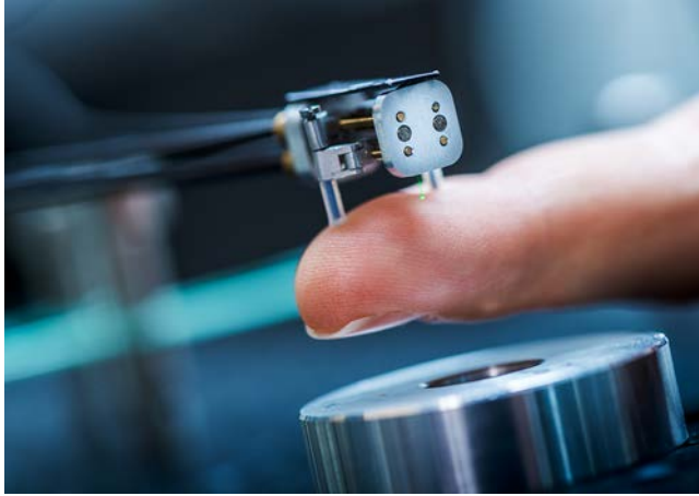
Robotic endoscope for minimal invasive laser surgery of bone (picture: F. Brüderli)
