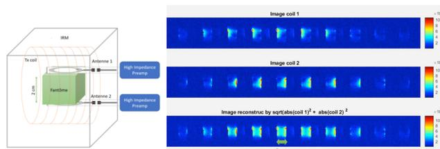
Figure 2: Decoupling performance assessed with MRI. A) Schematic showing two NMR surface coils facing each other, placed inside the MRI scanner and connected to our high-input impedance preamplifiers. B) Images obtained reveal minimal coupling between the two facing coils (image coil 1 & 2), despite their close proximity and potential strong coupling. The combined images allow to nicely depict the imaged phantom.
