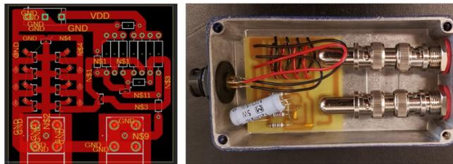
Figure 1: Above: Design and below: Construction (PCB design & integration) of the 2nd generation high-input preamplifier prototype.
