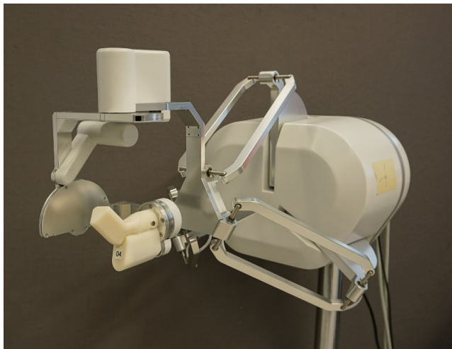
6-DoF haptic input device that can be used as a teleoperation master device. (Picture: Esther Zoller)
