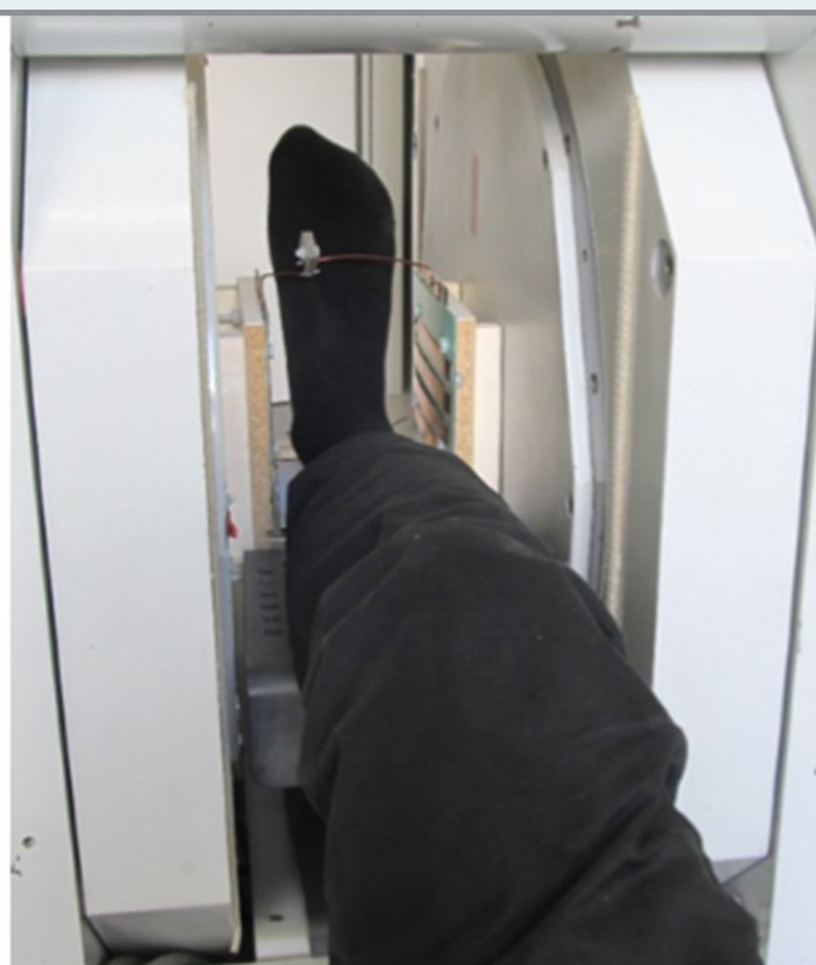
Left: open-access RF coil for flexible MRI and MR Elastography. Right: coil in a 0.1 T MRI for foot imaging.
