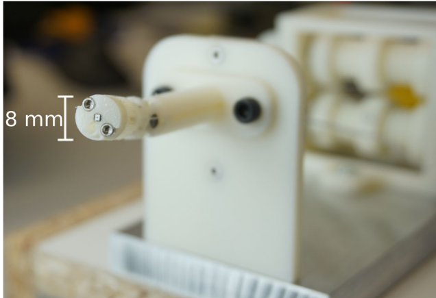
An endoscope prototype with an integrated miniature camera was built to track a target during arthroscopies. (Image: Stephan Schraivogel)
