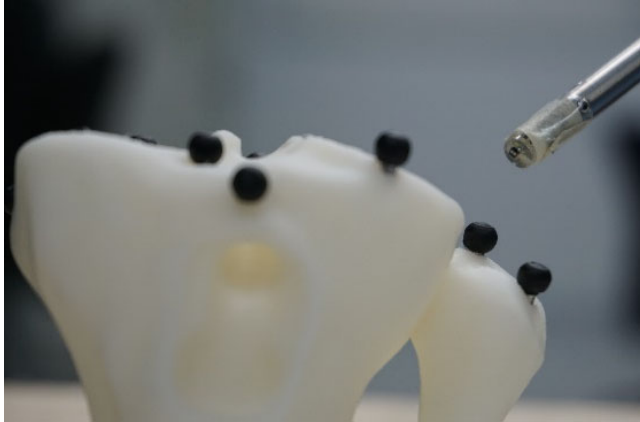
A miniature camera mounted to the endoscope's tip was used to estimate the pose of the endoscope relative to a knee phantom. (Mia Meyer)
