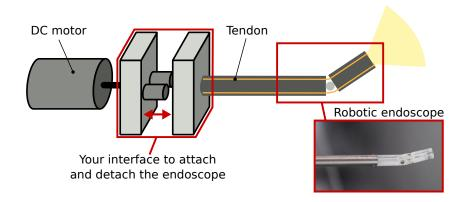
**Task description:** In this project, you will develop a "plug & play" interface that allows the surgeon to safely attach and detach the endoscope from the motors. This includes the following work packages:
