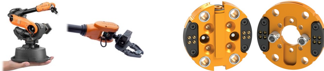
(a) Miniature 6 axis robot arm used in this project [2] (b) Example of an industrial miniature tool changer [3]
