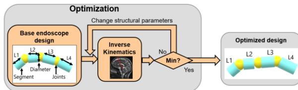
The optimization framework, where the algorithm provides the first guess, will take the first guess, use the IK, and calculate the cost function. Then the algorithm will determine if the structure is optimized or not. If it is not optimized, it will do the process again until the optimized structure is found. Created by: Omar Garrido
