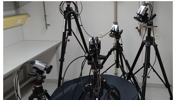
(b) An optical tracking system will be used to retrieve the positions of the markers in 3D space.
