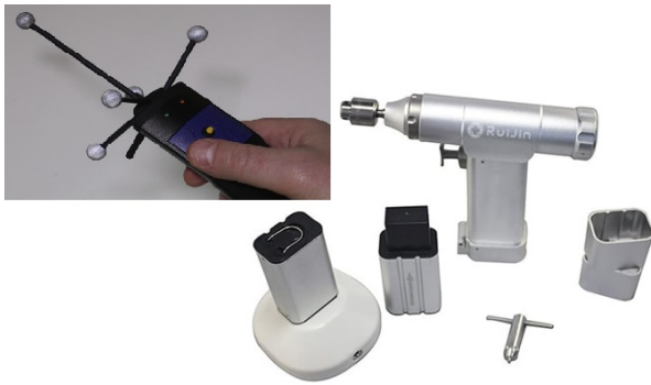
(a) A standard veterinary orthopedic drill ([3], bottom right) will be fitted with optical tracking markers ([4], top left).
