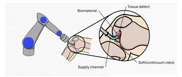
**Task description:** To develop a first functioning prototype of a flexible endoscope with a supply channel for the material dispensing tube.
