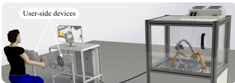
(a) The proposed micro-assembly system - the user side (left) consists of a range of human interface devices
