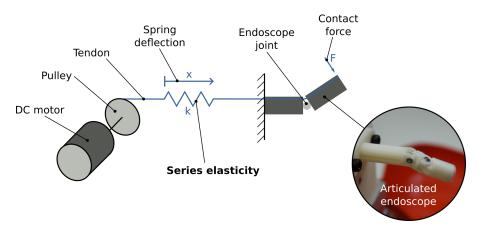
**Task description:** Recently, a robotic articulated endoscope prototype was developed at the BIROMED-Lab (Department of Biomedical Engineering, University of Basel). Thus far, two electric motors allow to control the endoscope via tendons in two degrees of freedom. Your task is to redesign the actuation of the endoscope, which includes:
