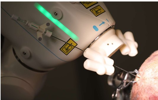
Figure 1: Head of the laser osteotome robot with attached biopsy needle guidance system and inserted biopsy needle.
