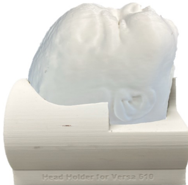
Figure 3. 3D-printed specimen holder that had been designed using a conventional computed tomography scan of the specimen with the matching 3D-printed replica of the specimen placed inside the holder.
