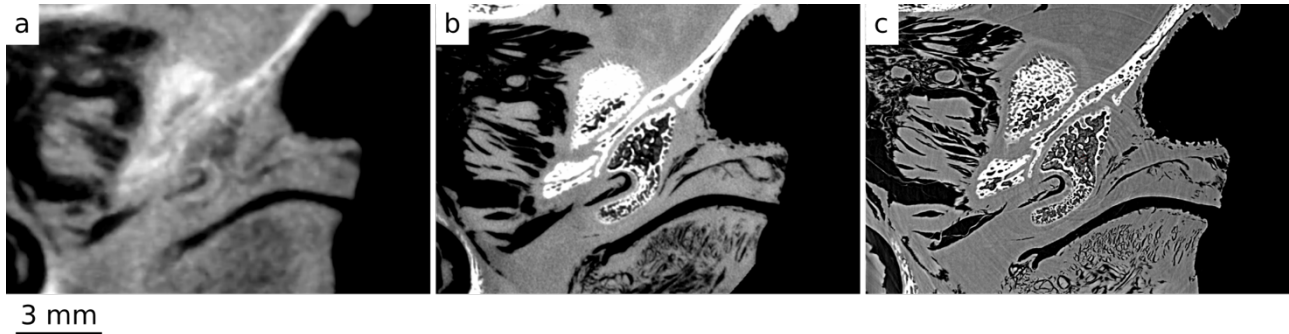
Figure 4. The hamular region imaged with the nanotom ® m (a), the Xradia 610 Versa (b), and the phase tomography at the synchrotron radiation facility (c).
