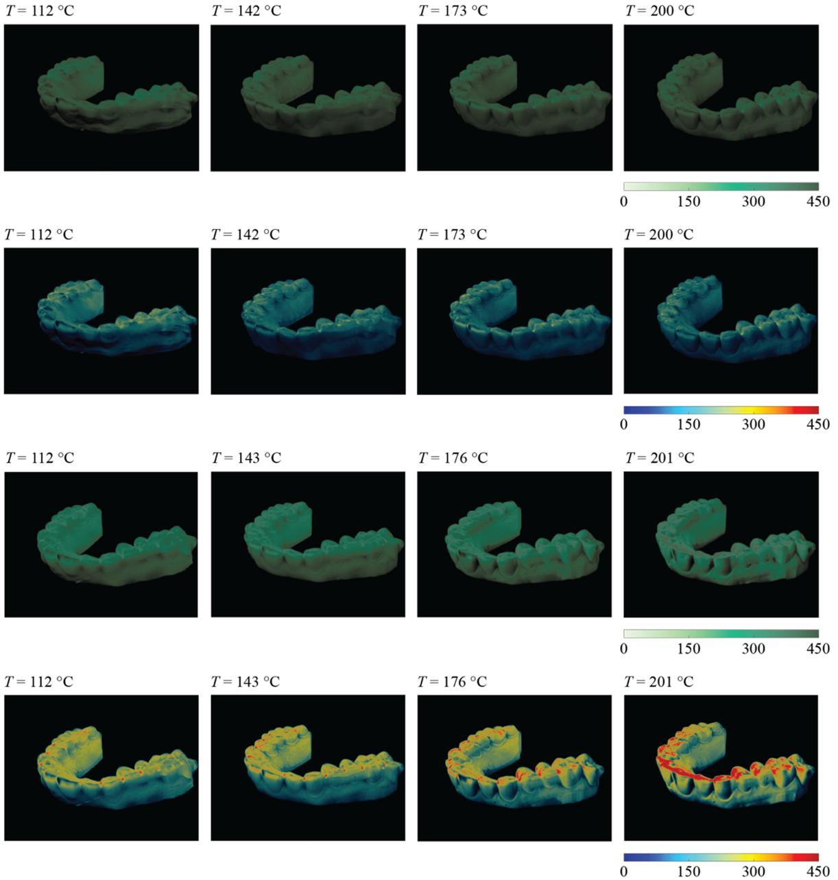
Figure 3. Color-coded aligner thickness distribution for the aligners NA.550, rows 1 and 2, and NA.750, rows 3 and 4. The color bars show the thickness in  $\mu\text{m}$ . The processing temperatures during the thermoforming are given as well.
