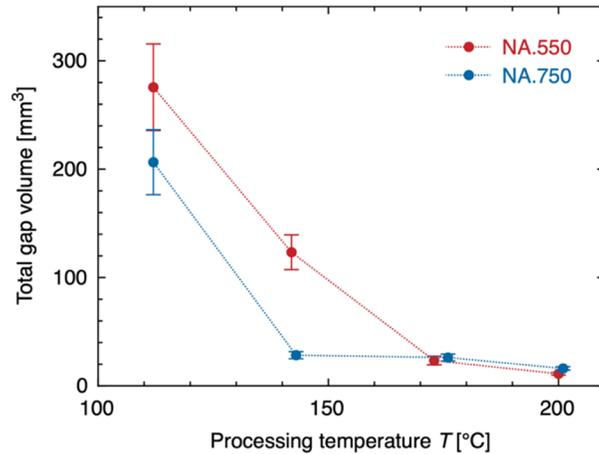
Figure 4. Total volume statistics for all gaps derived from the automatic method. The error bars were determined by using the three threshold values 140, 150, and 160. The dotted lines, which connect the data, should just guide the eyes.
