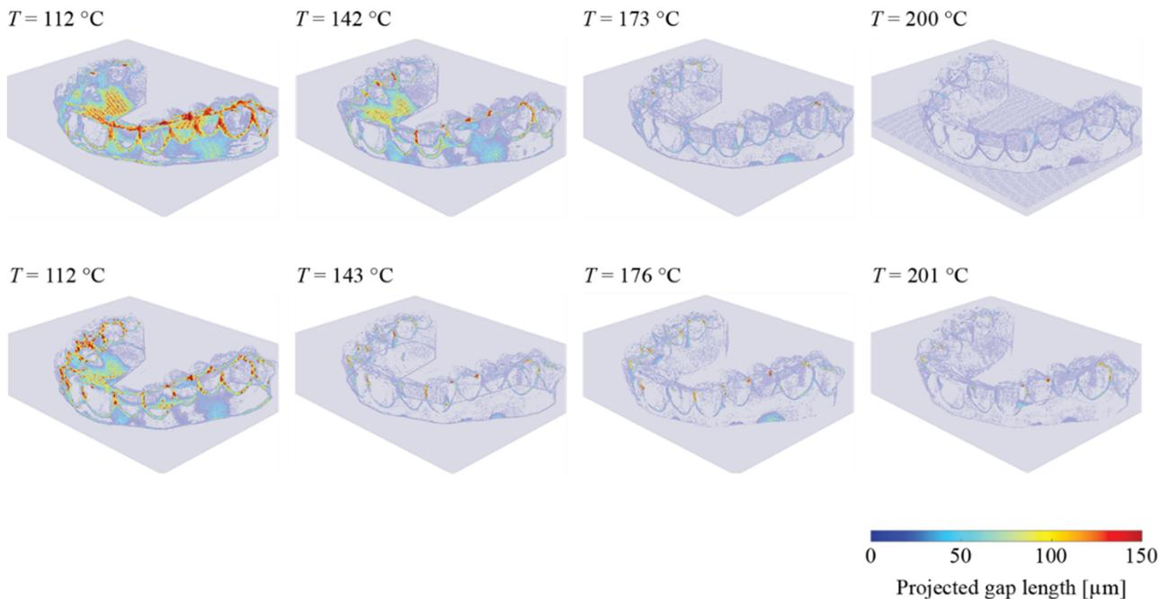
Figure 5. Rendering of projected gap lengths for the NA.550 aligners, top row, and NA.750 aligners, bottom row. The selected processing temperatures are indicated.
