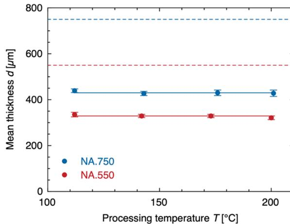
Figure 2. Thickness distribution of the mean when sampling 100 times 100 center-surface voxels, with solid lines showing the average value. The dashed lines show the thickness of the foils before thermoforming.
