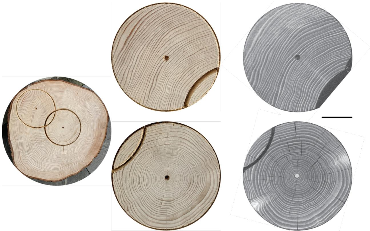
Figure 2. For the tomographic imaging using X rays, two cylinders with a diameter of 180 mm each were prepared, see photographs. The related tomography slices near the surface are represented on the right. The length bar corresponds to 50 mm.
