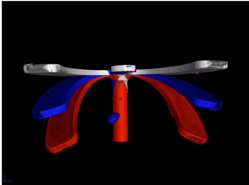
Video 6. The rotation of the assembly from the three tomograms perfectly demonstrates the gravity-induced bending of the silicone element. Its softness is characterized by a Young's modulus below 1 MPa.
