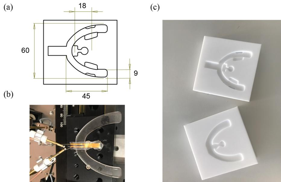
Fig. 2. The dimensions of the silicone elements for the current study are given in (a) and are comparable to the lateral size of the human oral cavity. The numbers represent the distances in millimeters. The photograph in (b) shows a two millimeter-thin silicone element combined with a pressure sensor contacted via flexible electrodes, as required for flexible electronics. The Teflon molds used are imaged in (c). For the present study the simpler mold was applied.
