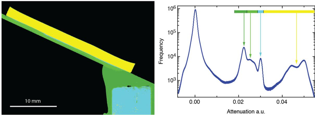
Fig. 4. The silicone element represented in yellow color within the virtual cut of the tomography data is supported by a polystyrene plate (lighter green), which is fixed on a polymer cylinder (bright blue) using a hot melt adhesive. The diagram on the right of the virtual cut is the histogram of the three-dimensional data with the color bar used for the visualization of the virtual cut. The silicone element seems to consist of two or even three differently dense components.
