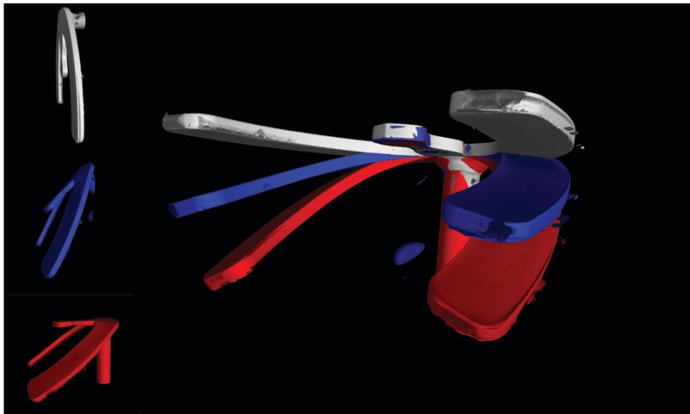
Fig. 5. The soft silicone element (silicone s, ratio 1:20) was imaged using the advanced CT-system nanotom<sup>®</sup> m in three orientations to the gravitation force; white – 0°, blue – 45°, and red – 90°. The assembly of the three tomograms clearly shows the impact of the gravitation force on the shape of the silicone element.
