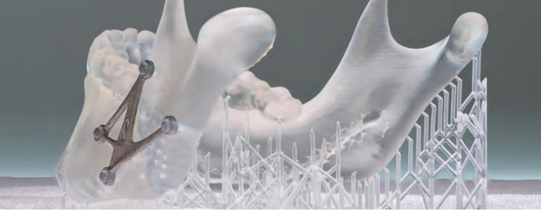
3D printed implant that stabilized a fractured jaw.
