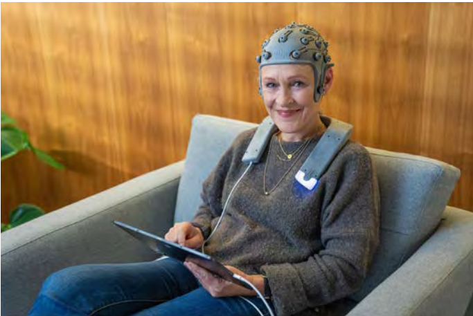
Figure 2: Patient specific, 3D-printed cap. The Miamind® Neurostimulator, registered with Swissmedic and MHRA, is tailored for each patient using 3D printing on the basis of MRI scans (picture: Bottneuro).
