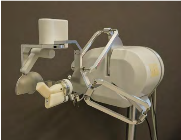
6-DoF haptic input device that can be used as a teleoperation master device. (Picture: E. Zoller)
