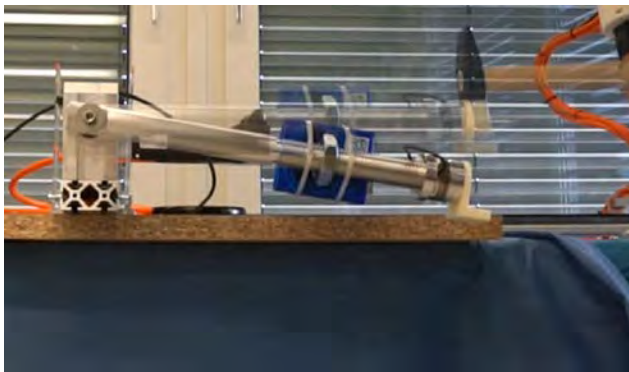
Impact test conducted with the testbench that shows the mechanical compliance in the joint (Picture: M. Karnam)
