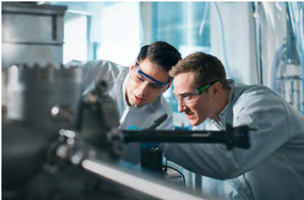
Master students working with a molecular beam deposition system to fabricate nanometer-thin polymer films used for artificial muscles, nanosensors and neural interfaces. (Picture: F. Moritz)
