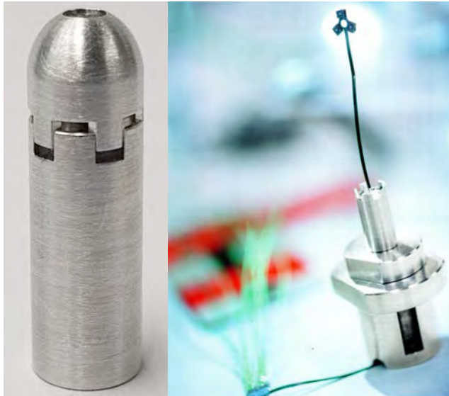
(a) Assembled encapsulated tri-axial force sensor for soft tissue palpation in neurosurgery (picture: Luca Marco Pavone), (b) Printed circuit board with the force sensors mounted on it - the core of the encapsulated force sensor (Picture: WSS/F. Brüderli/Longhini)
