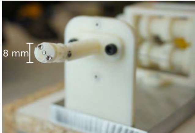
An endoscope prototype with an integrated miniature camera was built to track a target during arthroscopies. (Picture: Stephan Schraivogel)
