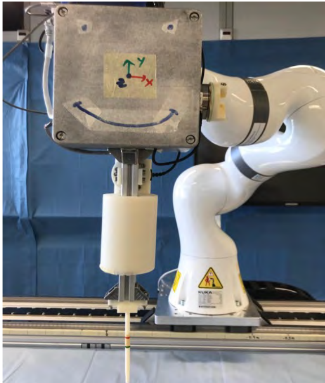
Figure 2: First prototype of handle aligned with the tool. This seems the most intuitive interface among the three that were tested.
