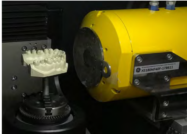
Figure 1: PEEK model on the rotation stage of the CT-system nanotom ® m (Picture: M. Sacher).
