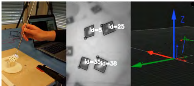
Figure 2: Pose estimation process (left to right): 1. acquire endoscopic images, 2. process the images to find the location of image markers, 3. estimate the pose of the endoscope relative to the anatomy (Picture: M. Meyer).
