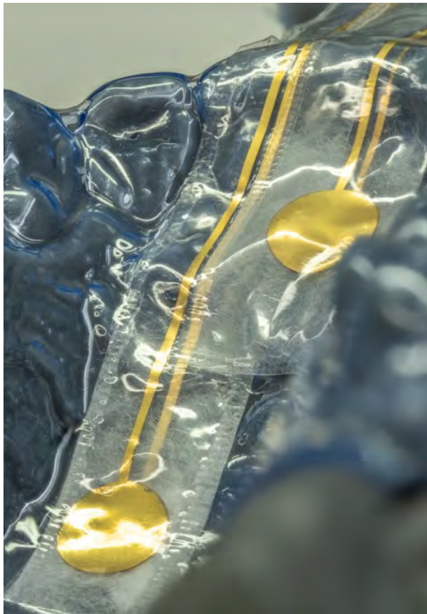
Figure 2: Two dielectric elastomer sensors embedded between two molded substrates for their integration/implementation into a personalized dental splint. (Picture: R. Wendler/DBE)
