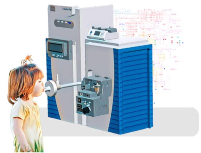
Figure 1: Real-Time Exhalation Maneuvre into Mass Spectrometric Platform (picture: Sinueslab).
