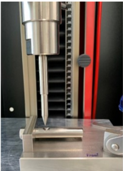
Figure 2: Set up of the fixtures created to perform the compression test with the Zwick Roell testing machine (picture: J. Sanjaume, regulated company).
