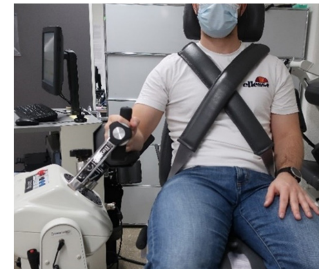
Figure 2: Biodex setup for shoulder external and internal rotation picture: Functional Biomechanics Laboratory, USB).
