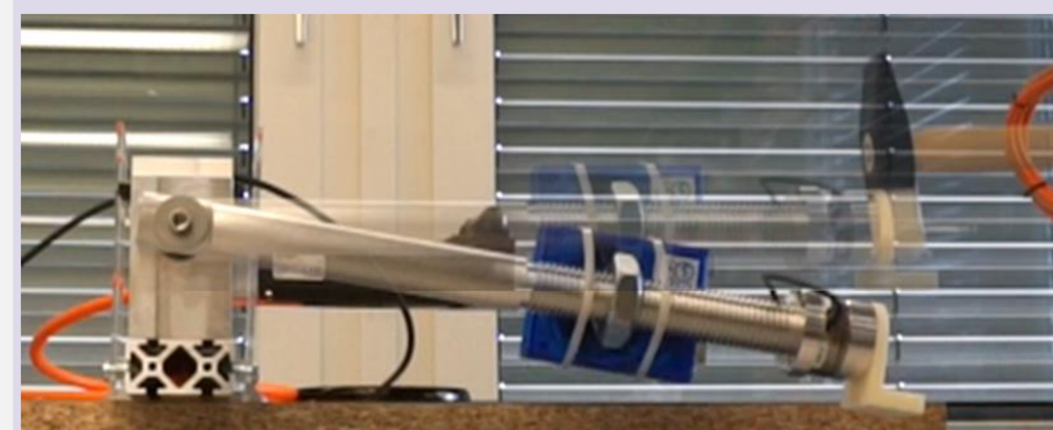
Fig: An SEA link that moved along the applied impact. It will return to its goal position (transparent) once the force is removed.
