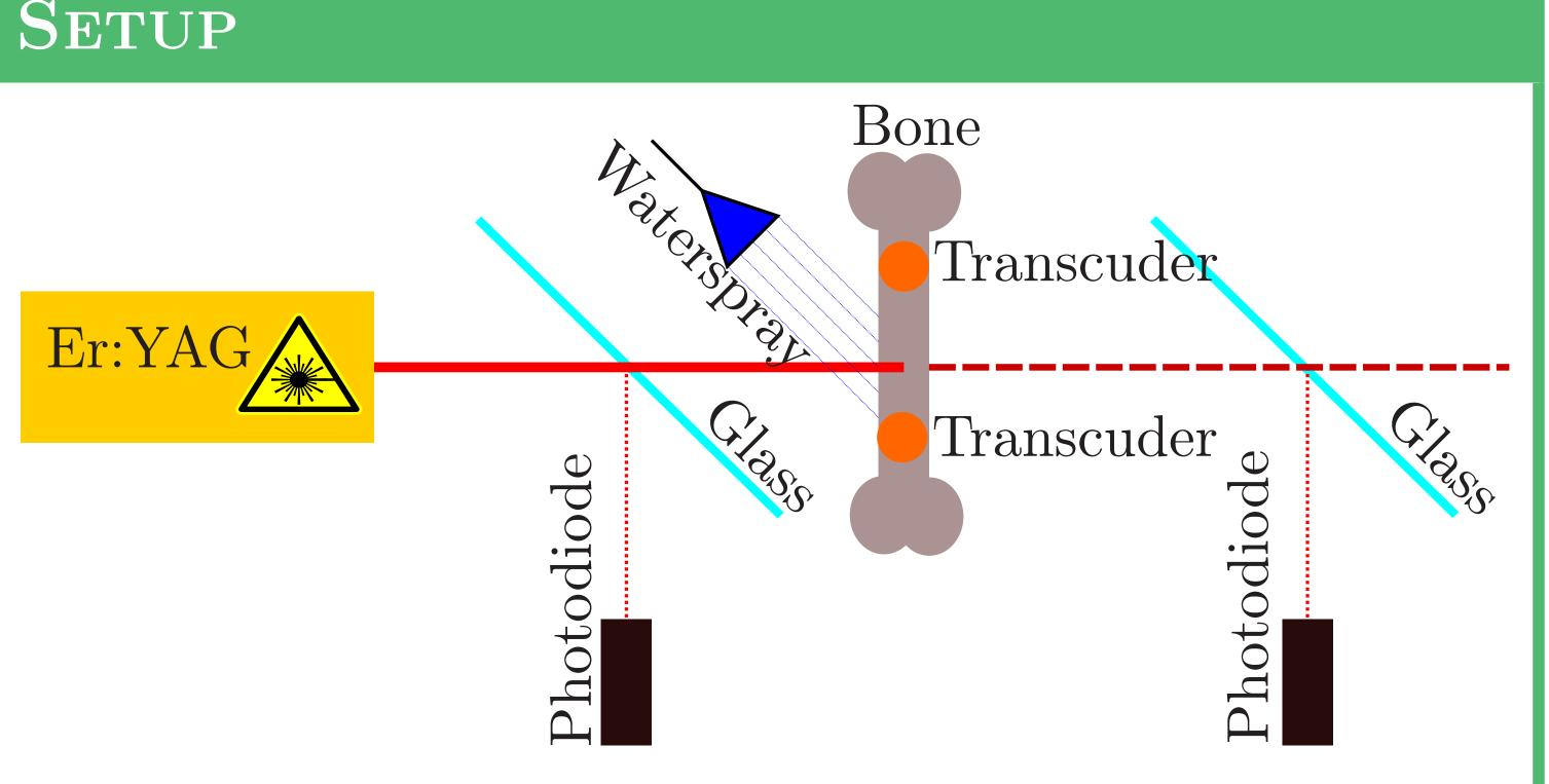
Transducer (Pico-Sensor) Er:YAG Laser
