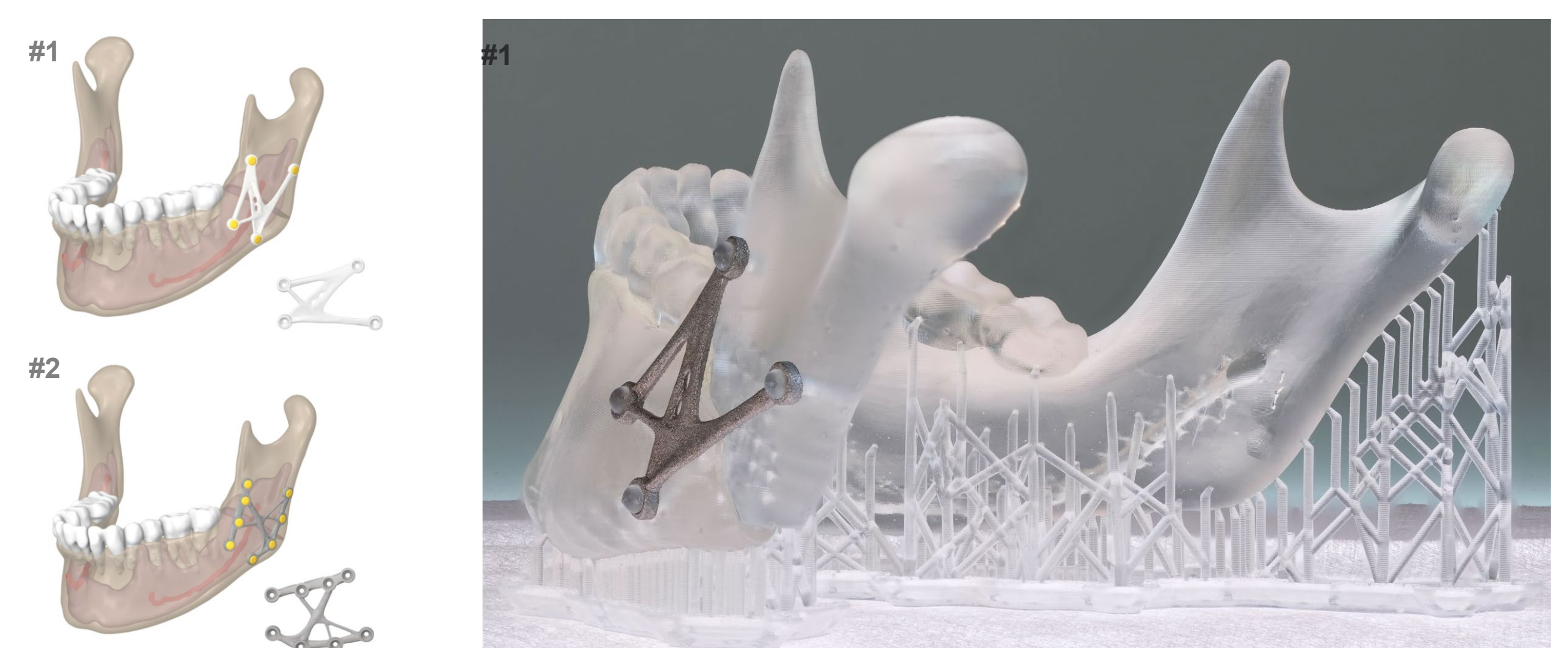
Figure 1. The implants generated with the topology optimization algorithm with four (#1) and eight (#2) screws and 3D printed implant-mandible model.
