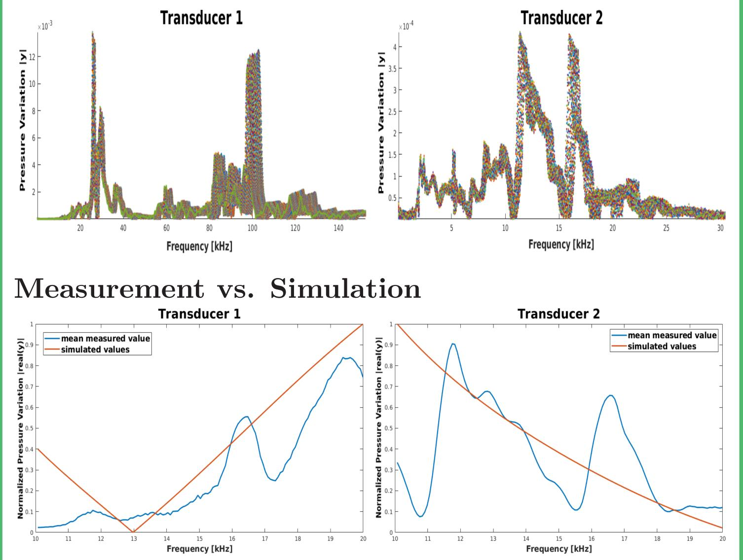
**Inverse Problem:** The acoustic waves generated by the laser ablating the medium will be used to reconstruct the structure of the bone and find depth of the laser-cut [2].
