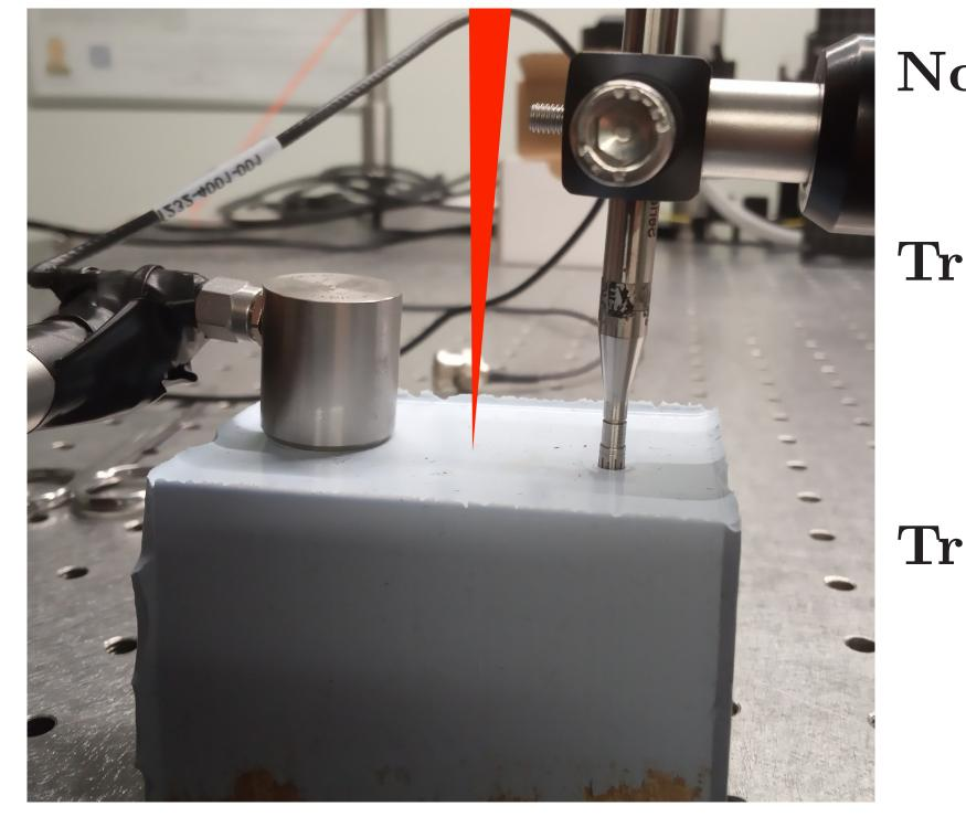
Nd:YAG Laser • 532 nm **Transducer 1:**
