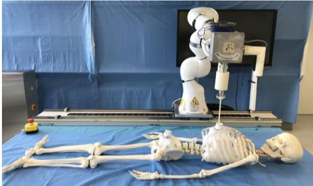
**Figure 1:** The user study setup with the macro-robot (7-DoF Kuka LBR iiwa) fixed via rails to the table and the mock-up skeleton with two trocars in front of it. Here the robot has two handles mounted that allow surgeons to move the tool as desired.
