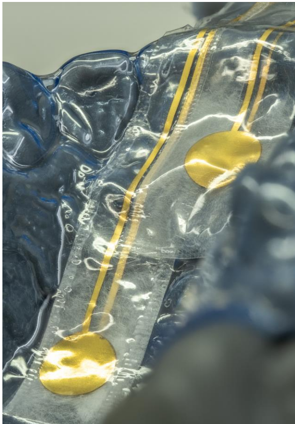
Figure 2: Two dielectric elastomer sensors embedded between two moulded substrates for their integration/implementation into a personalized dental splint. (Picture: R. Wendler/DBE)
