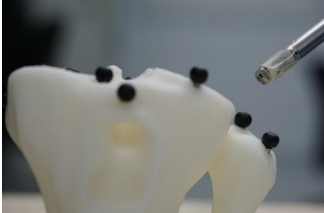
Figure 1: A miniature camera mounted to the endoscope's tip was used to estimate the pose of the endoscope relative to a knee phantom (Picture: M. Meyer).
