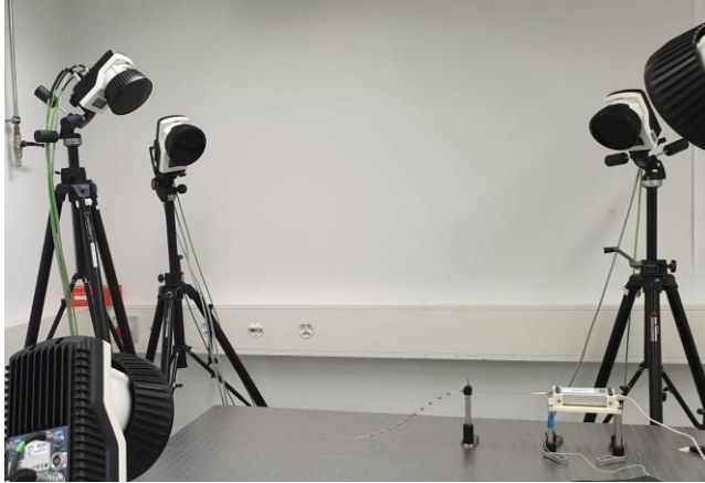
Figure 1: The experimental setup used for training data collection. The sensor's real shape and the edge-FBG spectrum were measured using a motion capture system and a fast spectrometer respectively (Picture: T. Renna).
