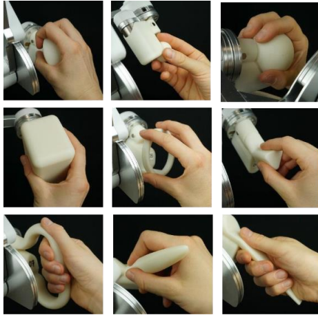
Figure 1: Nine different grasp type handles that can be mounted on the lambda.6 haptic device (Picture: E. Zoller).
