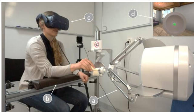
Figure 2: Experimental setup for the peg-in-hole task: a) lambda.6 haptic device (Force Dimension, Nyon, Switzerland), b) armrest, c) head-mounted display (HMD, HTC, New Taipei City, Taiwan), and d) the virtual environment that is displayed on the HMD to the participant (Picture: S. von Ballmoos).
