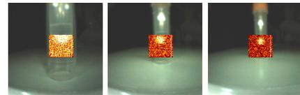
For each of the distances, the gamma activity image patch of the central pinhole is **overlaid on top of the optical image** of its camera.
