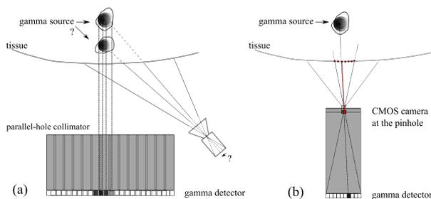
In order to overlay the two modalities, the pinhole and the camera need the same opto-geometric mapping and aligned viewing axes to produce a corresponding **perspective projection** (b). This cannot be achieved using an orthographic projection without knowing the depth of the source (a).
