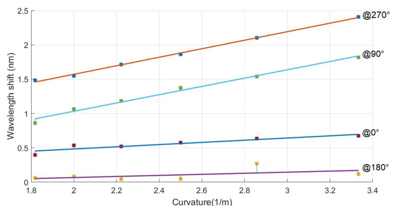
Fig 5: Bragg wavelength shift vs. curvature for different bending direction.
