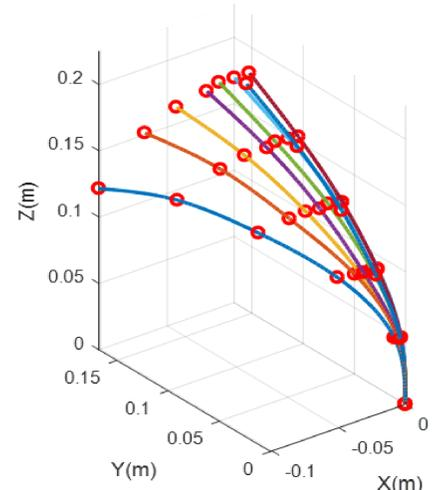
Fig 6: 3D reconstructed shape in different bending radii.
