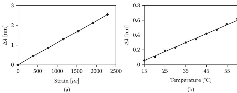
Fig 2: Typical wavelength-shifting response of an FBG to (a) strain and (b) temperature [2].
