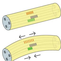
Fig 3: Expansion and compression while bending [2].
