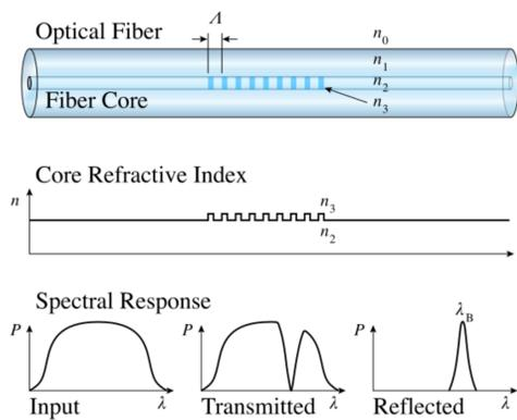
Fig 1: A Fiber Bragg Grating structure with refractive index profile and spectral response [1].
